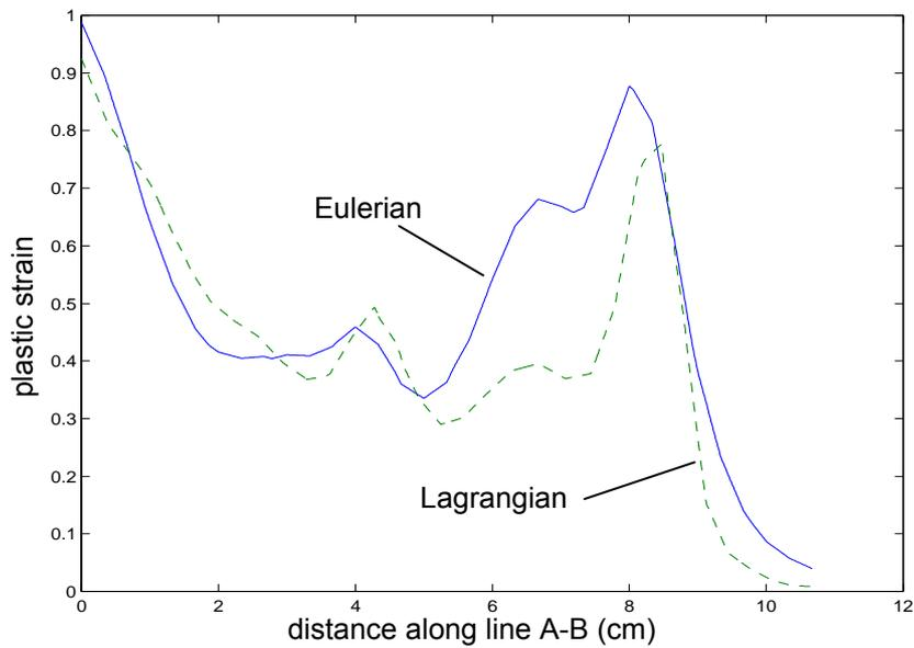
Figure 5. Effective plastic strain level at t=0.07s
