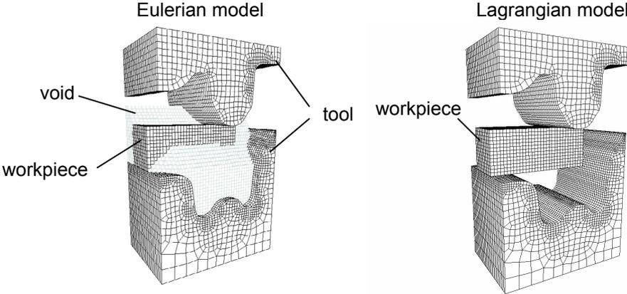
Figure 3. Eulerian and Lagrangian forging models
