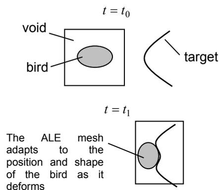
Figure 1. Moving ALE-mesh in impact simulation
