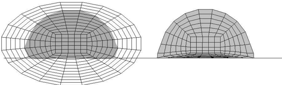
Figure 8. Material contours of impacting balls.
