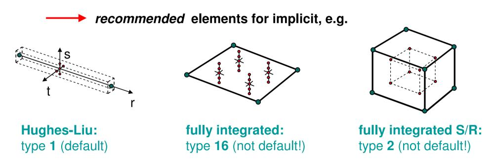
Alternate shell element formulations are substituted if requested elements are not available for implicit
